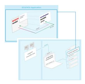
These simulation packages allow customers that use Bosch Motorsport control systems to simulate the functionality without using the hardware. These packages enable the user to run Bosch Motorsport and customer code area functions within the PTWin-Sim® environment.
